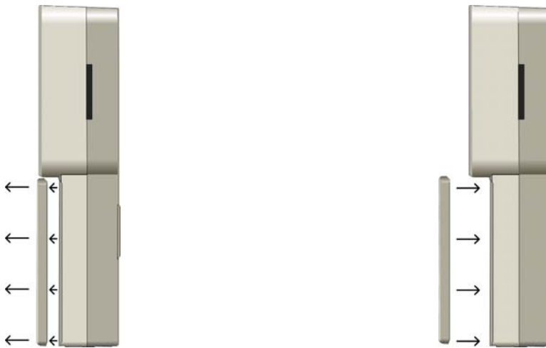
Figure 65 Removing the Front Cover
